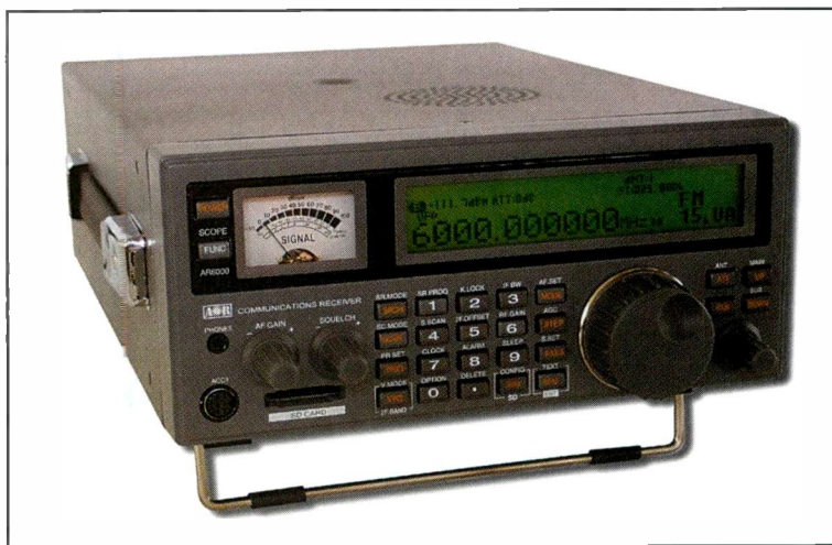
Photo A. The front panel of the new AR6000 shows the large tuning knob, keypad entry, LED display, and the ever-popular analog S-meter. (Courtesy of AOR USA)
