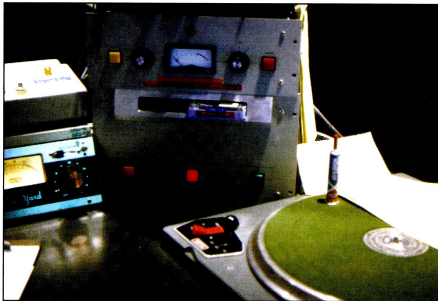
Photo H. Jan Lowry's long-ago snap captured KSRF's versatile Gates-brand monophonic YARD board, so called for its many channels and cross-switching options — as in a busy railroad depot's switching yard. This faithful piece of equipment served master control until "Tuesday, November 19, 1968," recalls Jan, "when KSRF(FM) went total multiplex stereo and inaugurated a new automation system. The first stereo broadcast was heard at 6 p.m. with the station's staff huddled around stereo speakers in the K-Surf general office area, attentively listening to the sounds of the surf' in magnificent stereo!" Also identifiable in this image is a Gates CB-77 turntable and Collins tape "cart" machine with record amplifier loosely resting on top. Check out the liberal use of plastic strip Label-Maker tape on the cart and cart machine. A common radio studio sight back in the day.
