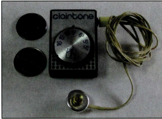
Photo C. This tiny Claritone two-transistor AM radio was popular in the early 1970s — a demonstration of AM radio's longtime portability. (Courtesy of Wtshymanski via Wikimedia Commons)
