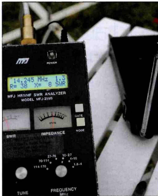
Photo C. At WB6NOA, the SWR measured lower than 1.3:1 on the Ventenna Quick Deploy HFp Antenna-at resonance.
