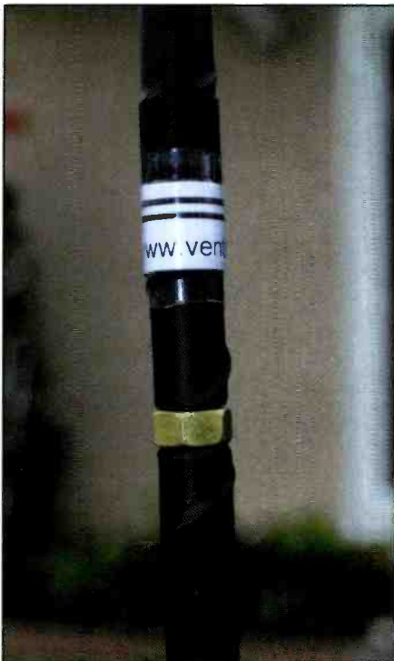
Photo F. This is the one-quarter-by-20 connection for each individual element.
