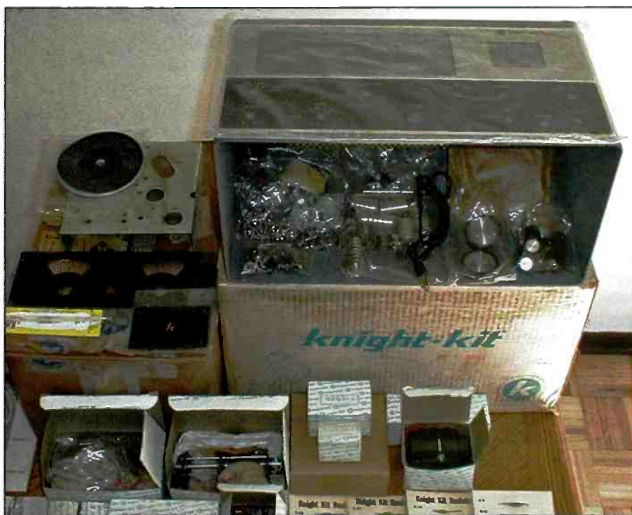
Photo D. "On the R-100A, the trimmer control was relocated below the meter and had a black knob with silver insert," K4NYW notes. The receiver was no one-evening project, as the parts count and packaging in this mostly-unopened kit shows.
