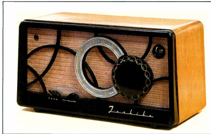
Photo E. Here's a classic AM-only radio, circa 1955, by Toshiba. This model 6SC-19 featured the popular and renowned five-tube superheterodyne circuit. (Courtesy of Masaki Ikeda via Wikimedia Commons)
