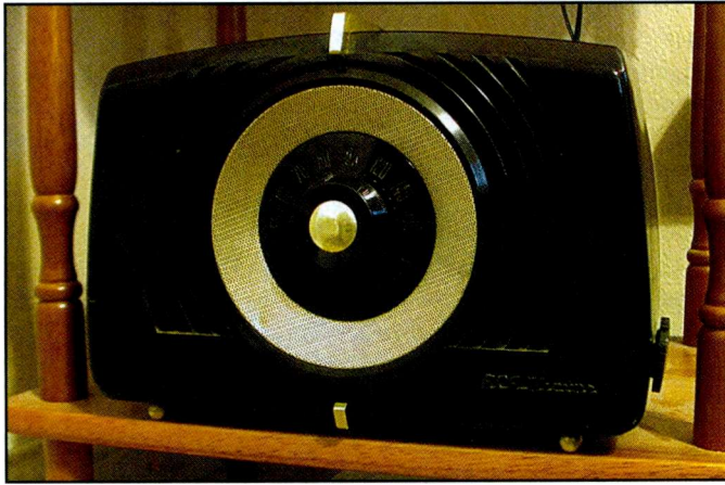
Photo J. This is the RCA model X-551 AM radio, circa 1952. It was typical of the post-World War II “All-American Five” tube configuration so popular at the time. (Courtesy of Wikimedia Commons)
