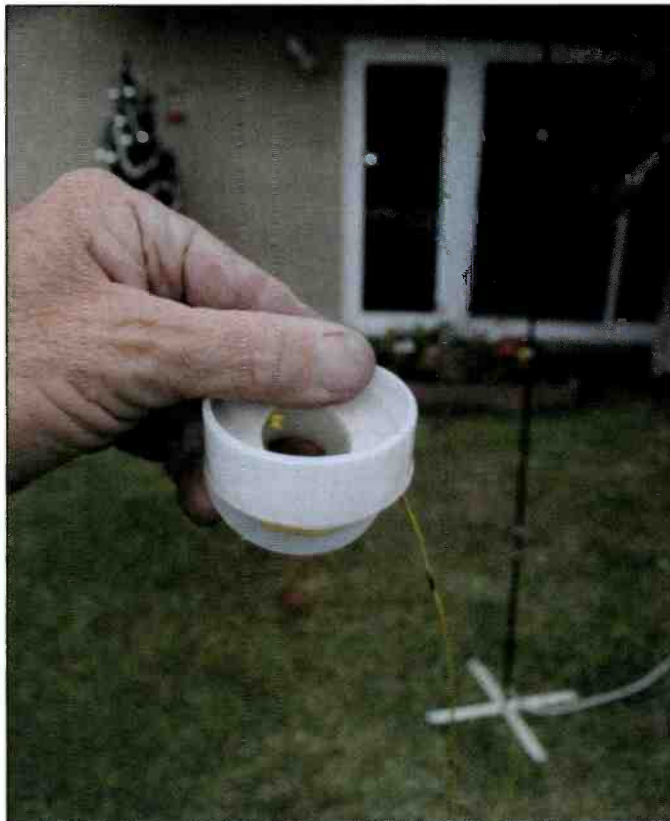
Photo B. Ventenna's HFp Antenna ground radials are pre-marked in black for each band.
